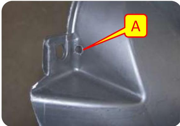
Once you have the rear trimmed to your liking, drill a 1/4" hole in the front of the inner fender. The hole should be in the corner of the front feature, roughly parallel to the stock hole [A].
