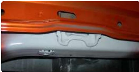
Cut off the Stock Flare Support Bracket. Paint any metal exposed by the cutting process with primer, clear coat, or a matching automotive grade paint. **IMPORTANT NOTE:** This is an optional step, but is recommended. The MetalCloak JK Overline Fender System will fit without removing the support bracket, however this bracket will become the limiting factor in your overall fender clearance.
