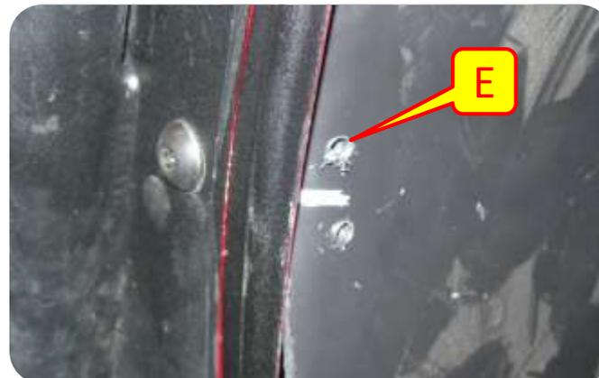
Double-check the fit of the inner fender at the rear and make any desired adjustments. Press the rear section into place and mark the locations of the two stand-offs on the inner fender piece; you can use the screw heads as a guide [D]. Drill two holes in these locations, about 1" from the edge, and about 1" apart (so the holes roughly align with the top and bottom of the stand-offs) [E].
