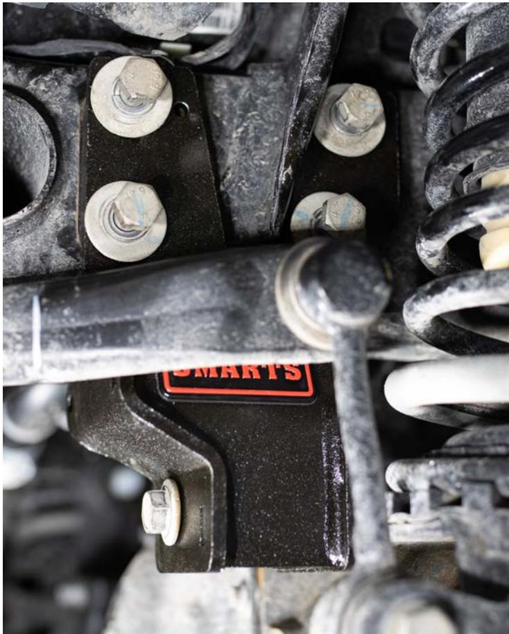
10. Use the 19mm socket and torque to the following spec (*for the steel box you can reinstall plug after torqueing*):
