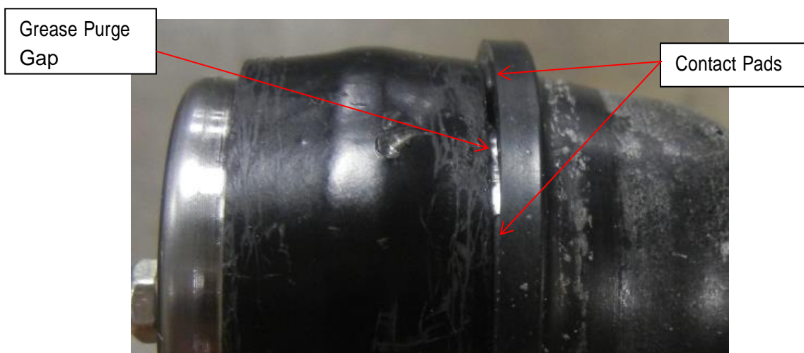
Figure 8: Properly Installed Seal Height
