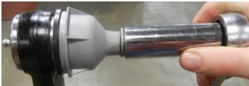
Figure 11: Torque Seal in Place
