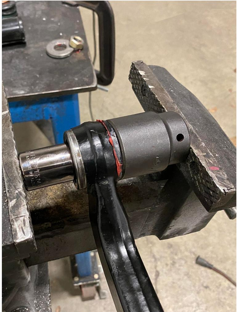
4. Press the boot seal on until the pads just begin to touch the machined face as shown below. **Do not over compress the boot seal as that will disallow the proper grease purging.**
