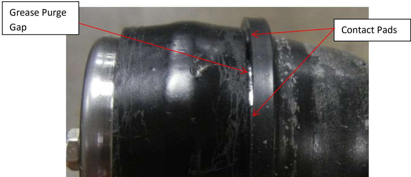
Once the replacement seal has been installed, you can now thread the tie rod or drag link end back into the linkage (if it was removed for install) and then reinstall the linkage and torque the nut to the Yeti XD linkage installation mandated torque specs.
