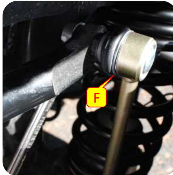
**Important Note:** MetalCloak recommends using red Loctite on each of the upper spindles of the sway bar end links.
