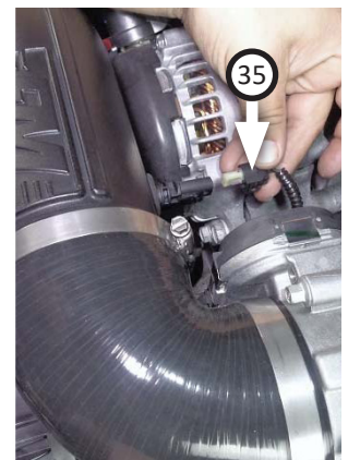
34. Connect air temp sensor extension harness (35) to vehicle's temp sensor plug. Route lead under coupler, connect other end to air temp sensor, then make sure all connections are secure.
