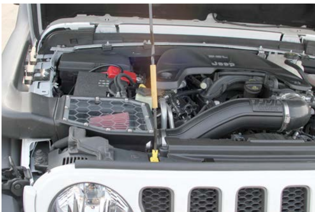
61. Make sure your snorkel airbox is properly sealed, then check all clamps at connections and ensure brackets are properly tightened.
