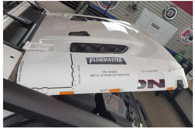
39. Open hood and set template onto it, aligning rear and side edges. Secure bottom edge with tape.
