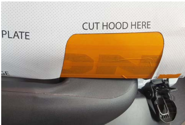
42. Lower hood onto snorkel tube and make sure template hood cutout is located correctly.
