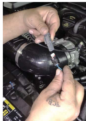
34. Connect air temp sensor extension harness (35) to vehicle's temp sensor plug. Route lead under coupler, connect other end to air temp sensor, then make sure all connections are secure.
