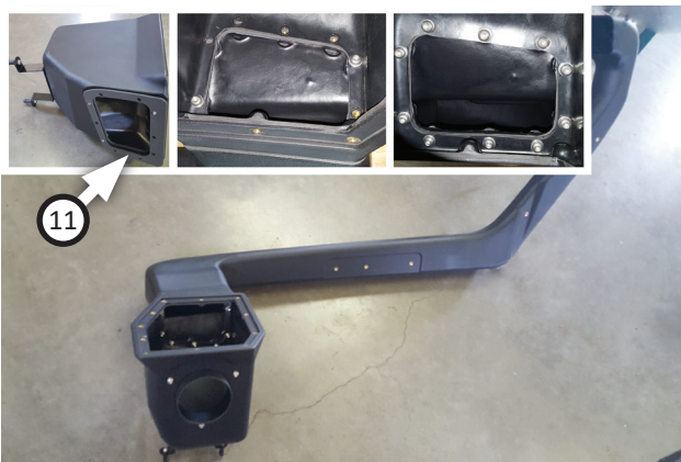
14. Connect airbox and snorkel gasket (11) to snorkel tube with (x10 ea.) screws (29) , lock washers (31) and flat washers (32) .
