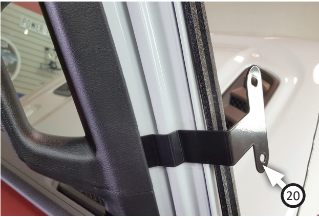
24. Place bracket 3 (20) over gasket and reinstall all grab handle components (removed steps 21-22).
