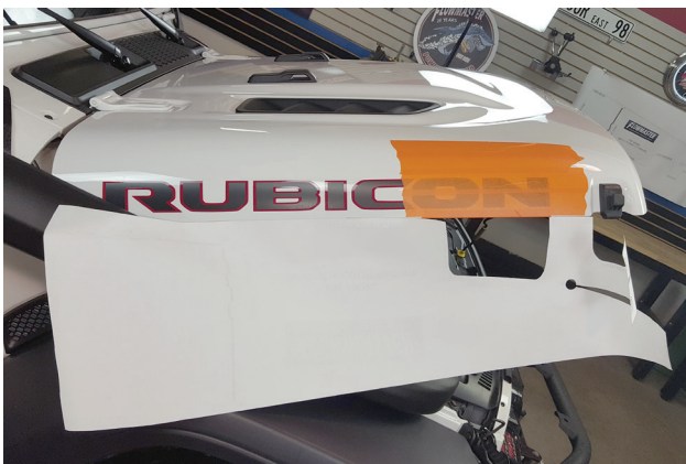
38. Fold template down off of hood then tape cutout as shown.
