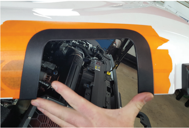
48. At this point, it may be better to work with a file to prevent cutting out too much material. The intent is to make adapter gasket fit your hood top layer as closely as possible, while centering it to snorkel tube (sides first then top).
