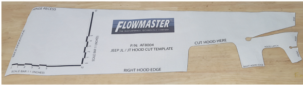
36. Carefully cut out paper hood cut template from kit. Be as precise as possible.
