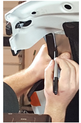
50. Open hood and set inner hood gasket (15) into bottom layer of cutout, then mark points that need additional cutting.
