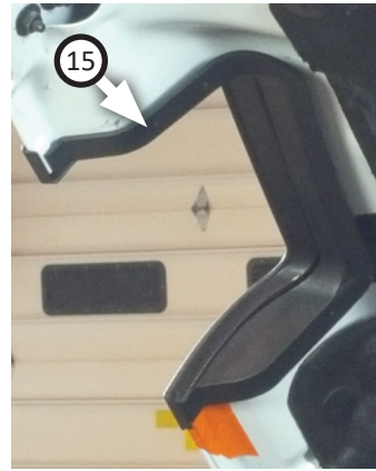
50. Open hood and set inner hood gasket (15) into bottom layer of cutout, then mark points that need additional cutting.
