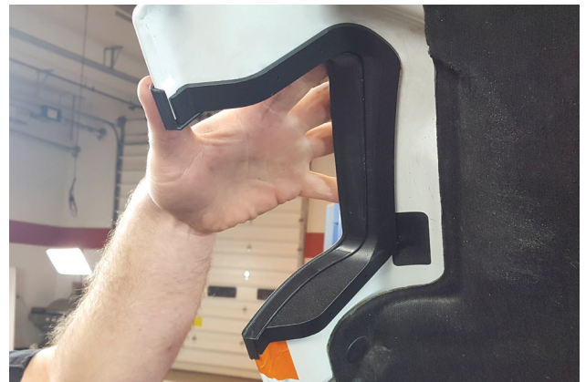
52. Once complete, your gaskets should fit together snugly without sliding around in cutout as shown.
