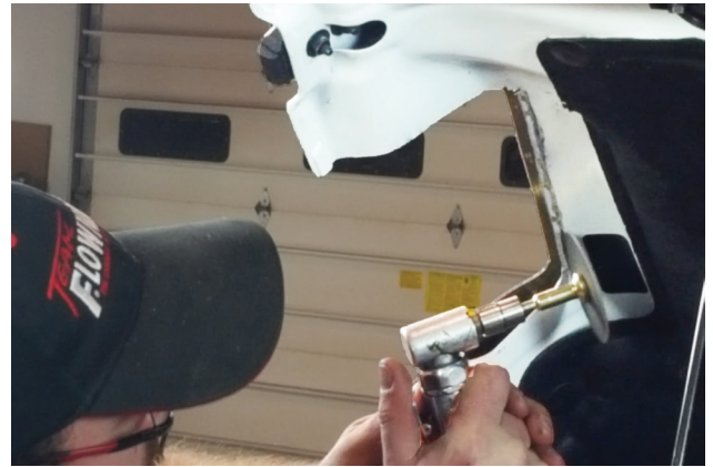
51. Cut out marked inner hood as necessary. Work slowly and carefully, checking cutout often until gasket fits exactly in place. Again, as you get close to fitment, work with a file to avoid excessive cuts.
