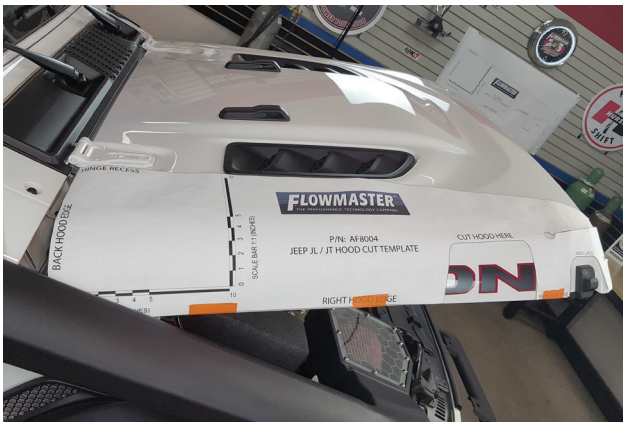
37. Open hood and set template onto it, aligning rear and side edges. Secure bottom edge with tape.
