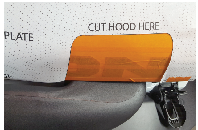
40. Lower hood onto snorkel tube and make sure template hood cutout is located correctly.
